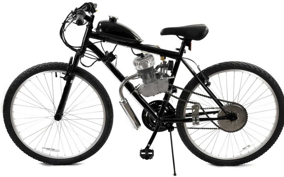
Figure 3: A "motor assisted bicycle" utilizing a gasoline motor [Source: https://gasbike.net/cdn/shop/products/gt5_pro_motorized_bike_1.jpg?v=1579577248 ]
