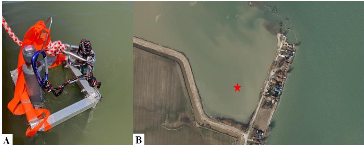
Figure 21: (A) Set up of deployed turbidity sensor. (B) Location of turbidity sensor in the Marsh.
