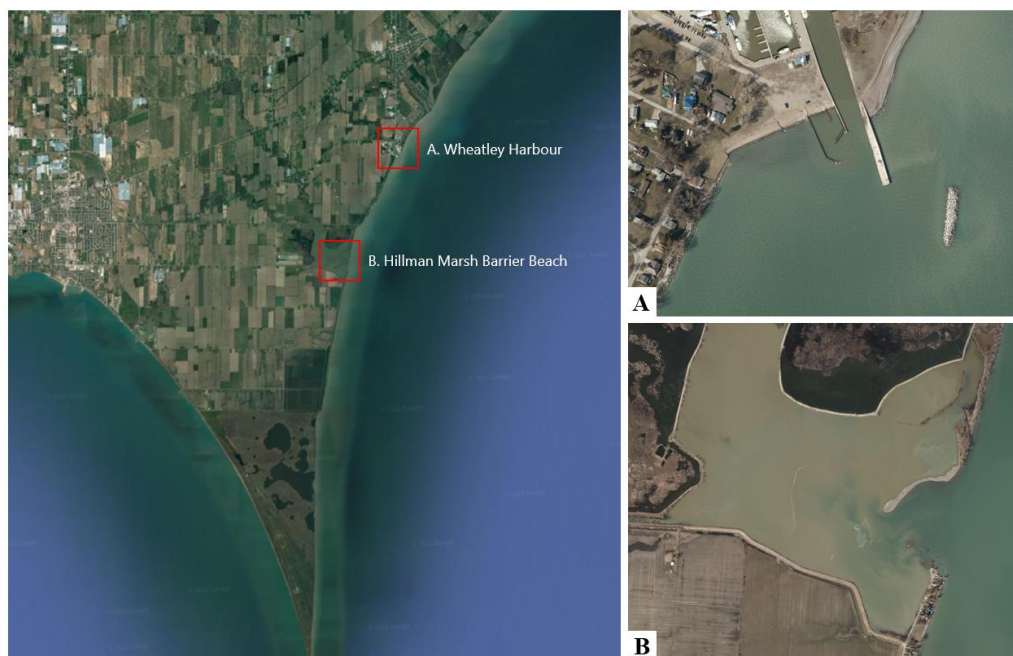
Figure 3: Hillman Marsh is located on the Point Pelee Peninsula, extending south of the shore of Essex-County. (A) The Wheatley Harbour and attached jetty have trapped or removed 525,000 m 3 of sediment from the downdrift shoreline, directly affecting (B) the Hillman Marsh Barrier Beach, a 1.5 km long, eastern-facing shoreline.
