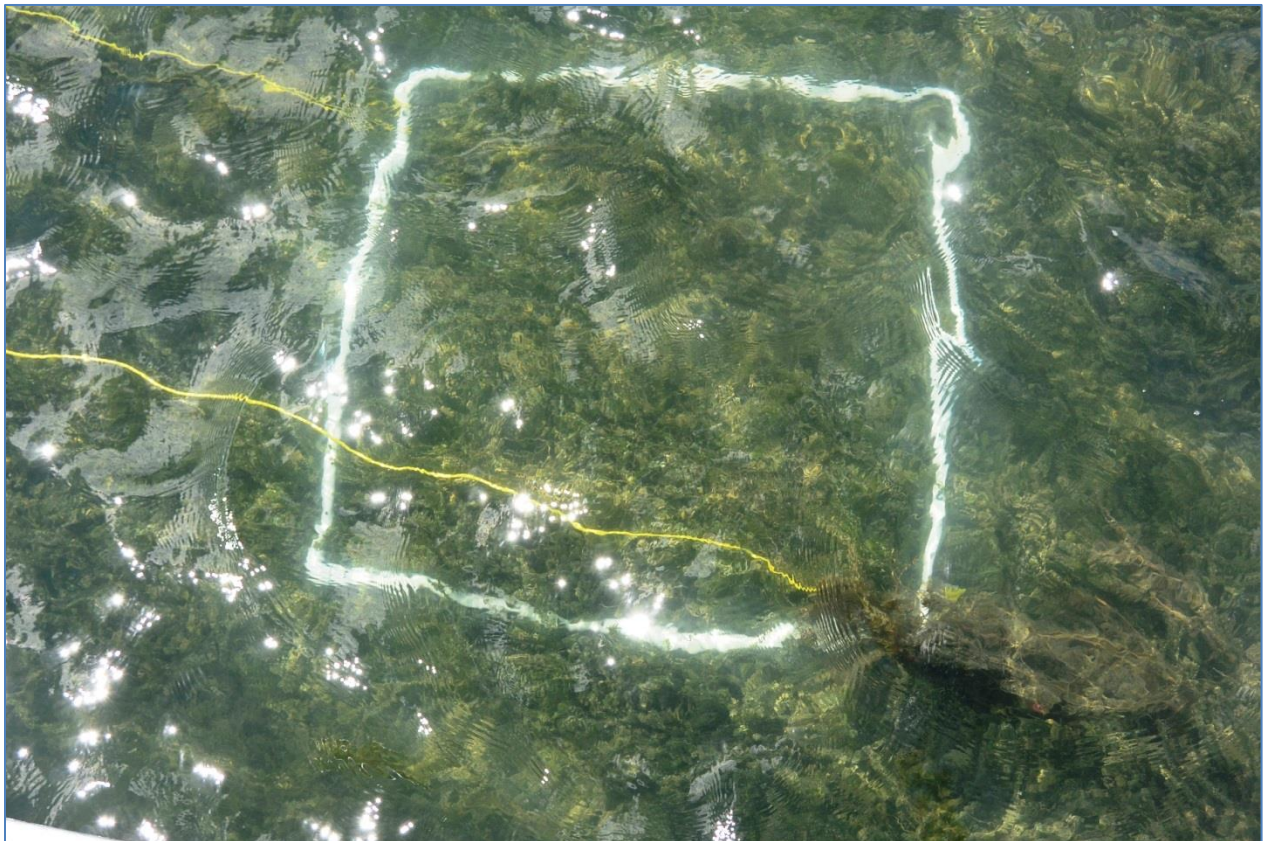
Figure 2: PVC pipe quadrat sampler, 1m x 1m, with attached floats used to sample SAV by rake method.
